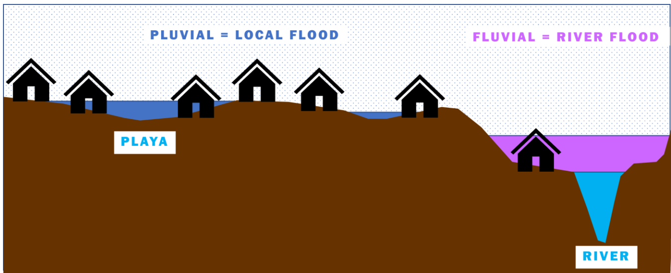
FIGURE 2-5 VISUAL REPRESENTATION OF PLUVIAL AND FLUVIAL FLOODING
